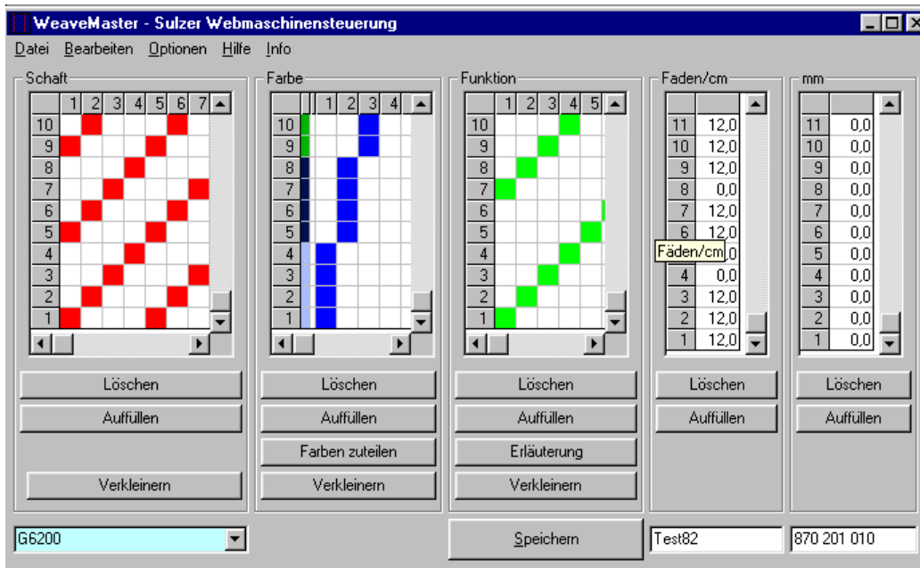
Figure30: Machine control Sulzer weaving machines:
